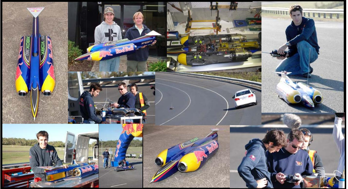
Rick, a keen and talented modeller in his own right, sought the assistance and guidance of Model Engines' technical guru Neil Addicott to help set up the Twin turbines in the car and program the Multiplex Evo 9 transmitter. The receiver used was a Multiplex 7 Channel Synthesised Dual Conversion Receiver, servo's were all Hitec Digital's and suspension parts were mainly sourced from GV.
