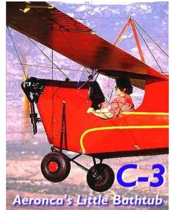
The fuselage was quite bulky as it needed to be wrapped around the aforementioned pilot and as the engine was mounted so high and the propeller was so tiny there was no need for a long undercarriage and indeed it looks like it was connected directly to the fuselage. That must have resulted in an atrocious ride over rough ground or on less than perfect landings.
