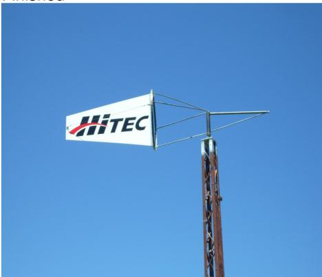
Model Engines have supplied us with a smaller Multiplex windsock so I have made a 4 metre high post that is hinged at the base so that the windsock can be replaced at ground level. This windsock is located beside the directional mustang and now it will be much easier and safer to glance sideways to see wind direction when landing, rather than looking back to the original windsock.
