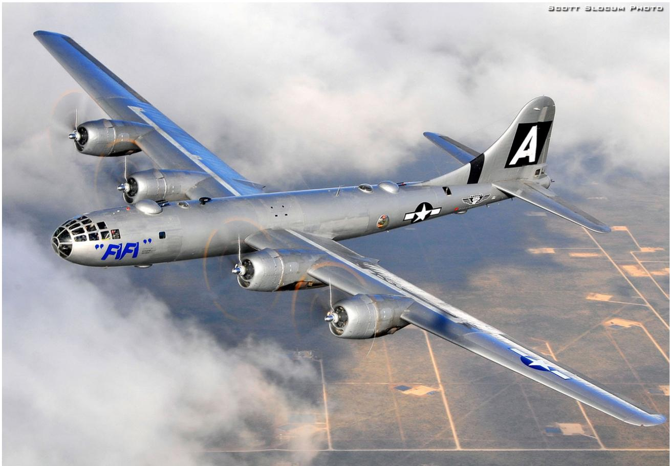
A major advance was that it was to be pressurized which avoided the crippling cold and oxygen mask breathing which the B-17 and Lancaster crews had endured at bombing heights.
