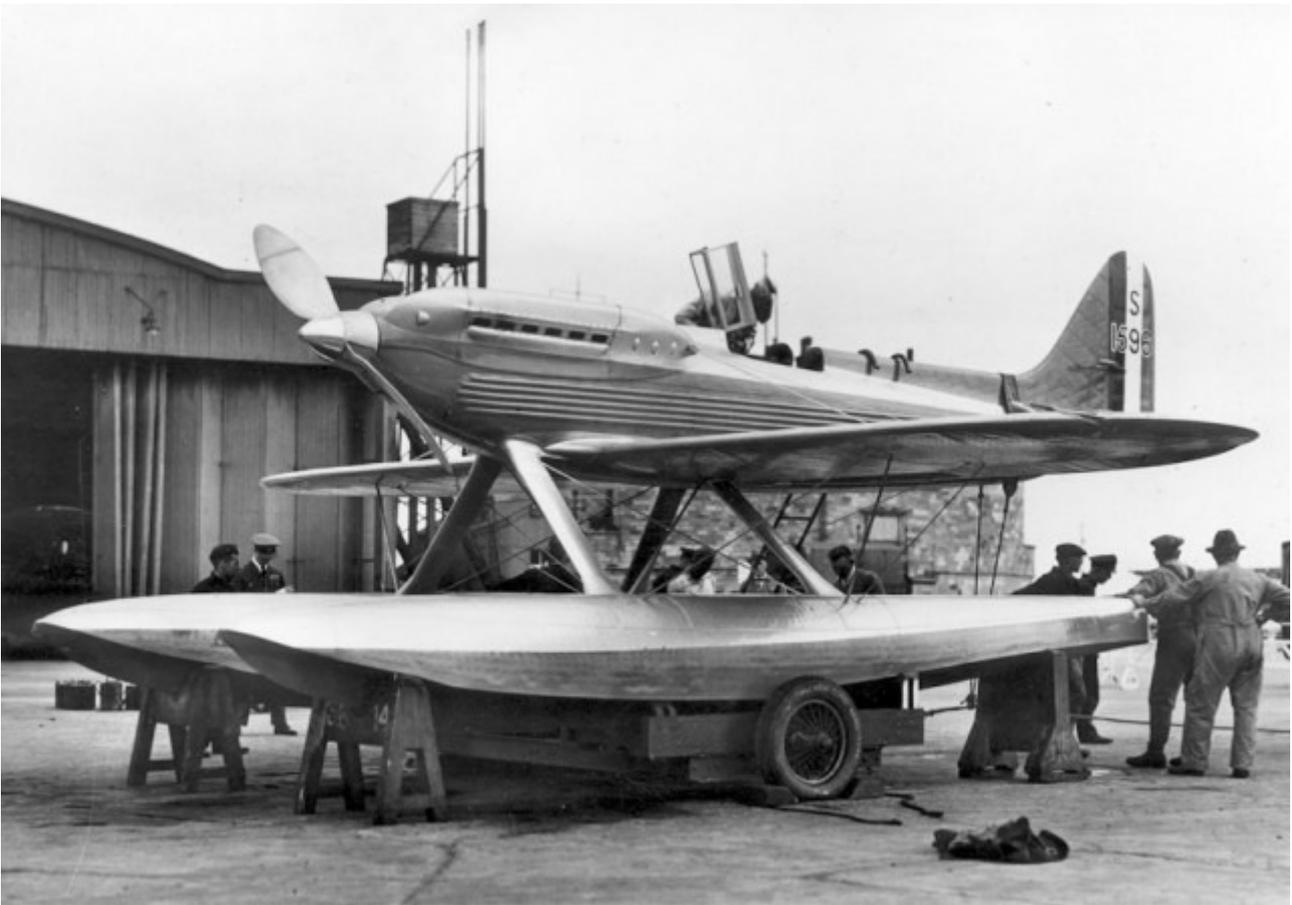
Note the pitch of the propeller, ( not providing much thrust for take – off , but a high top speed )
