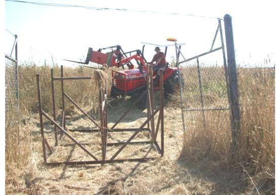
The forklift tine unit being used to lift and tow a scrap frame from the windmill / dam area
