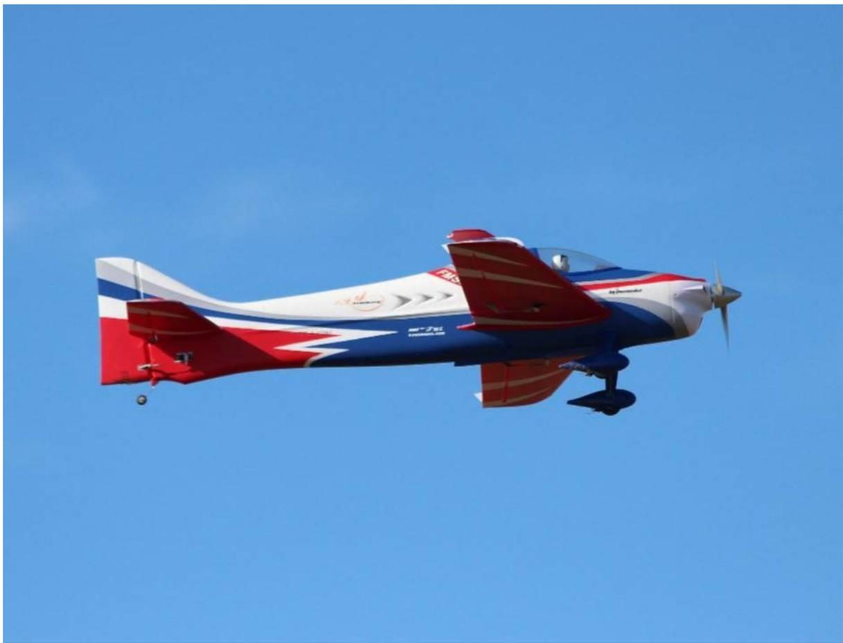
Daniel Jenkins FMS Olympus F3A model, EPO foam, 425KV motor, 6S LiPO, 1400mm wingspan
