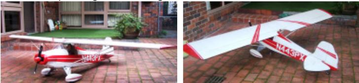
2. Yak 55 90" (2.286mtrs) span aerobatic aircraft fitted with 85cc Stihl petrol engine with new CH Electronics spark ignition system.
