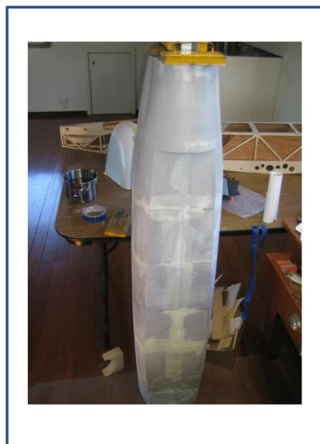
They used a 3 view to make a 3D software model using 3D software which Andrew is very good at manipulating. He then "cut" it up into sections and then is in the process of 3D printing them with Ivan putting them all together to create the plastic "plug". Ivan is doing the wing design on normal CAD which will be covered with G10 when built.
