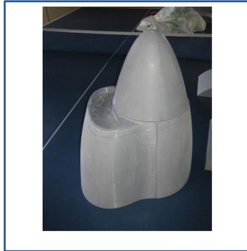
Looks like Andrew and Ivan are up to building strange models again. Several strange plastic parts have been seen at the field as they accumulate stuff for their new model. Turns out they are building an F-86D Sabre about 2M long. They are in the process of making a plug and will then make a mould and then make fibreglass fuselages and then build normal "built up wings".
