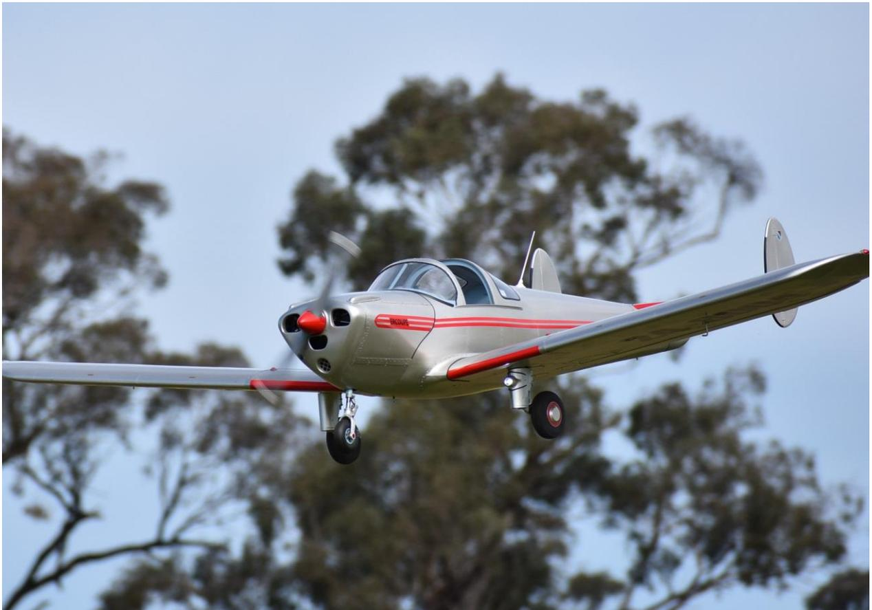
This nice Ercoupe from Tim Dehann was built from a 1/3 scale Balsa USA kit. Tim added many scale details to the basic kit and has modelled it on a full size Ercoupe which is based at Tyabb Airport. Power is via a Saito FG-61TS four stroke petrol engine, and the radio system is a Spektrum DX18. As you can see from the photo, Tim has done an outstanding job on the model.
