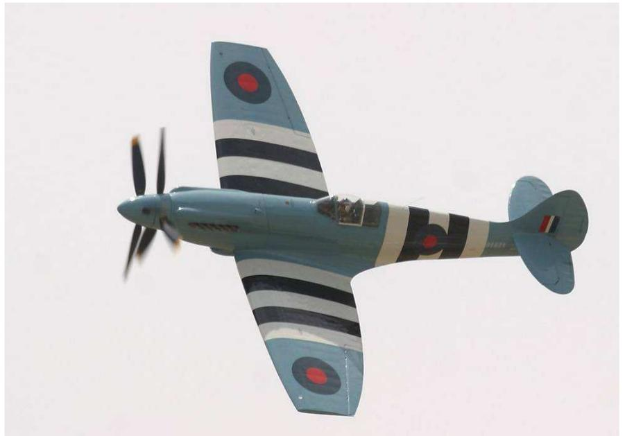
Up to five propeller blades were needed to absorb the power of the Griffon and in one of the greatest visible changes to a Spitfire some variants were fitted with two contra rotating three bladed propellers!
