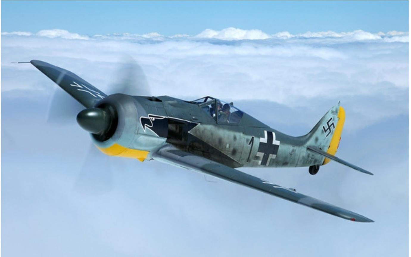
A lack of turning ability was due to the relatively small wing. That small wingspan however led to more speed and greater maneuverability. Its pilots loved it, finding it much easier to fly than that other great Luftwaffe fighter, the Me 109. In particular the wide undercarriage made landing much easier. An extraordinary number of Me 109s were lost in landing accidents.
